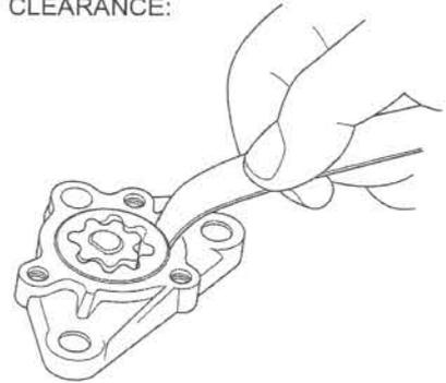
Measure the side clearance using a straight edge and a feeler gauge.
