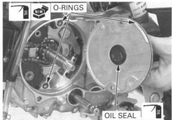
*Be careful not to damage the oil seal lips* Install the stator base and tighten the screws securely.
